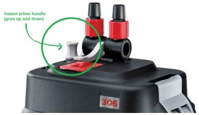
Once you hear water being drawn into the unit, return the instant-prime handle to the down position. Air will be expelled through the output nozzle, causing the water in the aquarium to bubble. Once the bubbling in the tank stops, you will know the air is out of the system, and the reservoir is full. Plug the power cord into an electrical outlet and the pump should start immediately.
